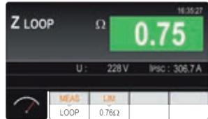
测量回路阻抗 Loop impedance
